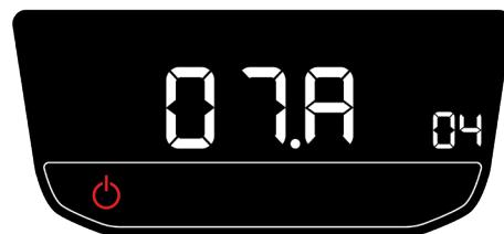
After a few seconds, it will enter initial configuration mode in order to select maximum unit power between 1.2 (1230 W) or 2.0 (2020 W) from the control panel. Select the required option with the up or down buttons on the panel or remote control and confirm by pressing the ON/OFF button on the unit.
