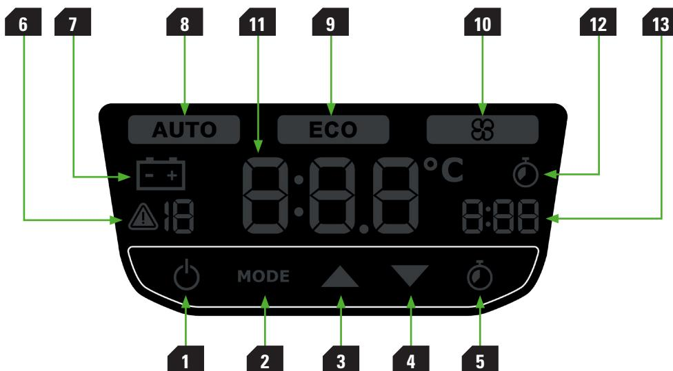
**1 ON/OFF:** Unit On/Off button. Pressing once turns the unit on and leaves it ready for operation. Pressing again turns the unit off.
