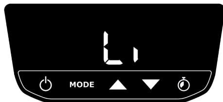
The user must select the measurement scale, either degrees Celsius ( $^{\circ}\text{C}$ ) or degrees Fahrenheit ( $^{\circ}\text{F}$ ), in order to complete the configuration. Select the required option using the up or down buttons on the control panel or remote control and confirm with the ON/OFF button on the unit. After this last confirmation, the unit will go off and remain ready to power up.
