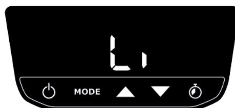
To complete the settings, the user must select the temperature measurement scale for the cooler, in either degrees Celsius (°C) or Fahrenheit (°F). Select the required option using the up or down buttons on the control panel or remote control, and confirm with the cooler's ON/OFF button. After this last confirmation, the unit will switch to "Stand by" mode and remain ready to power up.
